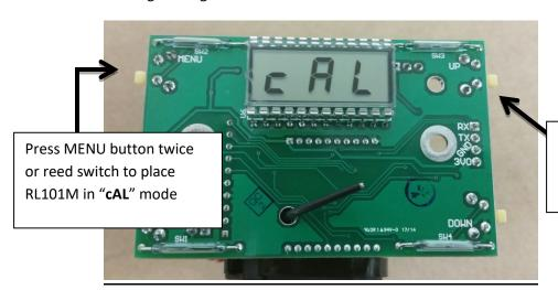
Use the Up button to automatically calibrate the sensor to 2.5 %
