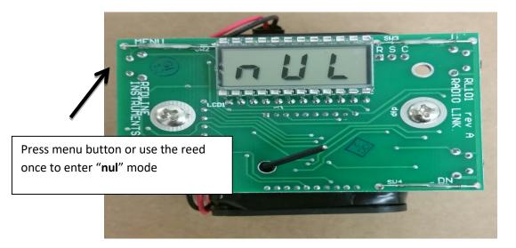
To place the RI101 into NULL Mode press MENU button our use the magnet with the reed switch once "**NUL**" will flash on the display. The RL101 Head unit monitors the gas level but does not send messages when in **NULL** Mode. NULL Mode is used removing any errors in the amplifiers that may cause a gas reading when there is no gas. Use the Up or Down buttons to adjust the readings to zero.
