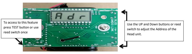
To access to this feature press TEST once, "**Adr**" will flash on the display when in that mode. Use the UP and Down buttons to adjust the Address of the Head unit. There must be a corresponding address set in the Monitor.
