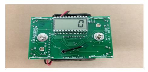
The RL101 Head unit monitors the gas level. If the gas level is greater than or equal to the background setting, the unit will send a message every 5 seconds; if less than the background setting, the unit will send a message every 5 minutes. When the Rl101CB is in normal mode it will display a zero.
