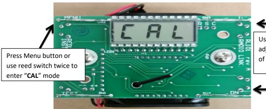
Use the Up and Down buttons to adjust the reading to match the value of the calibration gas
